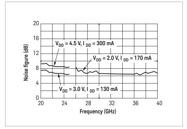
Figure 7. Noise figure vs. frequency
