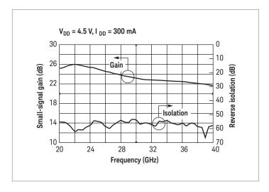
Figure 2. Typical gain and isolation vs. frequency<sup>1</sup>
