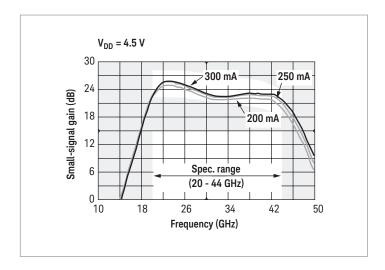
Figure 15. 1GG6-4066 broadband gain as a function of drain current vs. frequency with VDD =  $4.5\,\mathrm{V1}$
