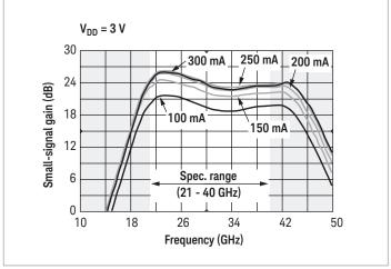
Figure 5. Broadband gain as a function of drain current vs. frequency with  $V_{DD} = 3 \ V^1$
