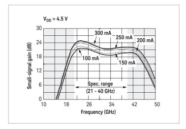
Figure 4. Broadband gain as a function of drain current vs. frequency with  $\ensuremath{V_{DD}} = 4.5 \ensuremath{\,\mathrm{V11}}$
