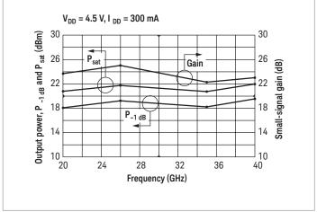
Figure 11. Output power and gain vs. frequency characteristics  $^{2}$
