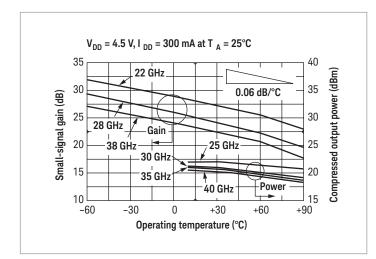
Figure 6. Small-signal gain<sup>1</sup> and compressed power<sup>2</sup> vs. temperature
