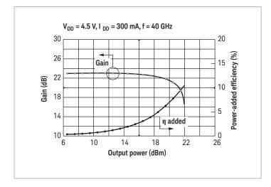
Figure 10. Gain compression and efficiency characteristics<sup>2</sup>
