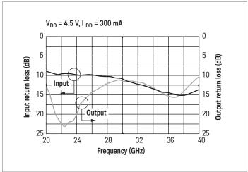
Figure 3. Typical input and output return loss vs. frequency<sup>1</sup>
