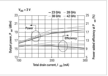
Figure 9. Output power 1 and efficiency vs. drain current with  $V_{DD} = 3 V$
